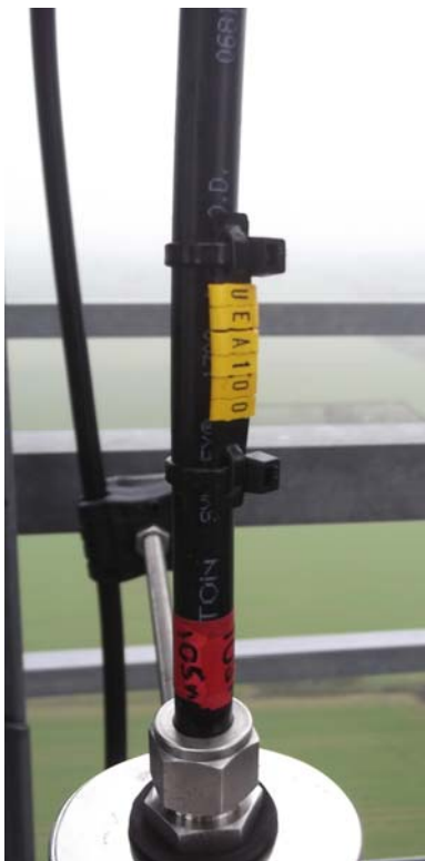
Figure 2: The 100 meter line installed in the tower at Tacolneston. The attachment of the air sampling line to the stainless steel cup is shown on the left and two of the air sampling lines running down through cleats is shown on the right.
