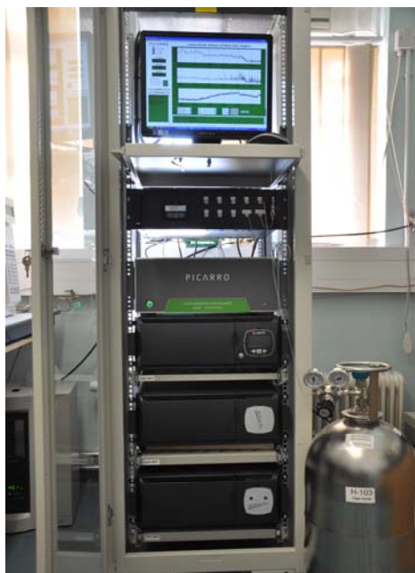
Figure 29: The Picarro in the centre with sample module above and the monitor, showing real time urban measurements, at the top of the rack unit. The bottom three units is the uninterruptable power system which prevents instrument shutdown in case of a power cut.
