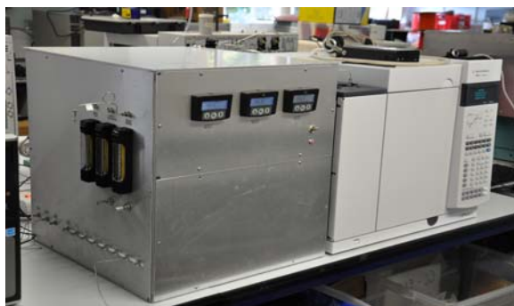
Figure 28: The Ridge Hill instrument built to measure N 2 O and SF 6 .
