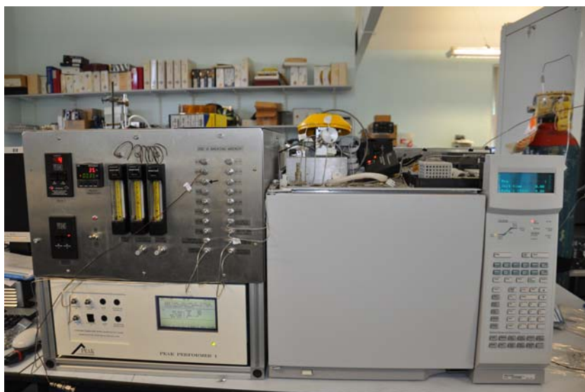
Figure 26: The Tacolneston multiple detector which makes measurements of N_2O , SF_6 , H_2 and CO .
