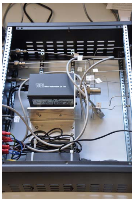
Figure 27: The sample module for delivering air from different tower heights and calibration standards to the Picarro.
