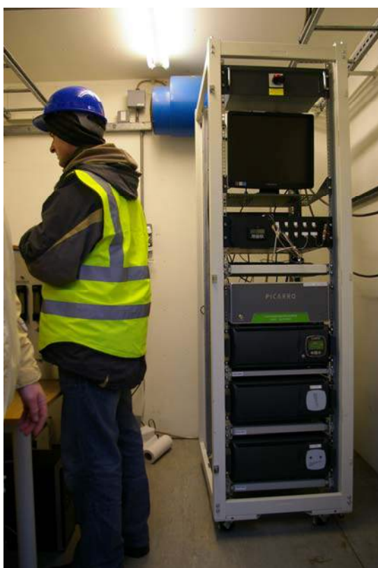
Figure 5: The Picarro installed in the cabin at Ridge Hill with backup power system below (left) and the sample module and Picarro in close up (right).
