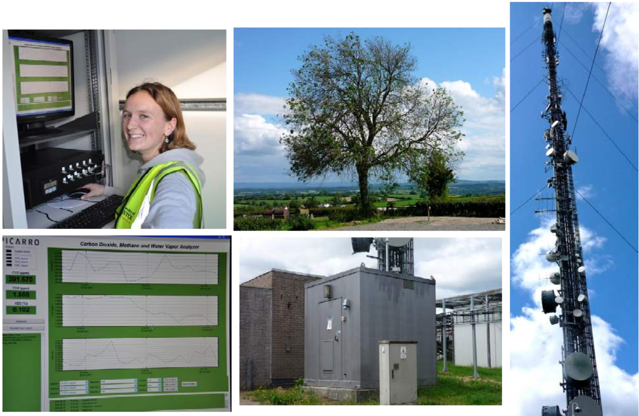
Figure 3: The 166.4 metre Tall tower at Ridge Hill (right) with a view of the surrounding countryside (top centre). The grey cabin houses instrumentation and the images on the left show the first measurements of CO 2 and CH 4 taken from the new site at Ridge Hill.
