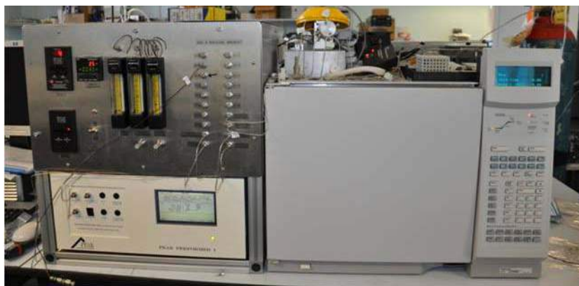
Figure 6: The TAC-MD which simultaneously measures SF 6 and N 2 O on the ECD (to the right) and CO and H 2 on the PP1 (bottom left).
