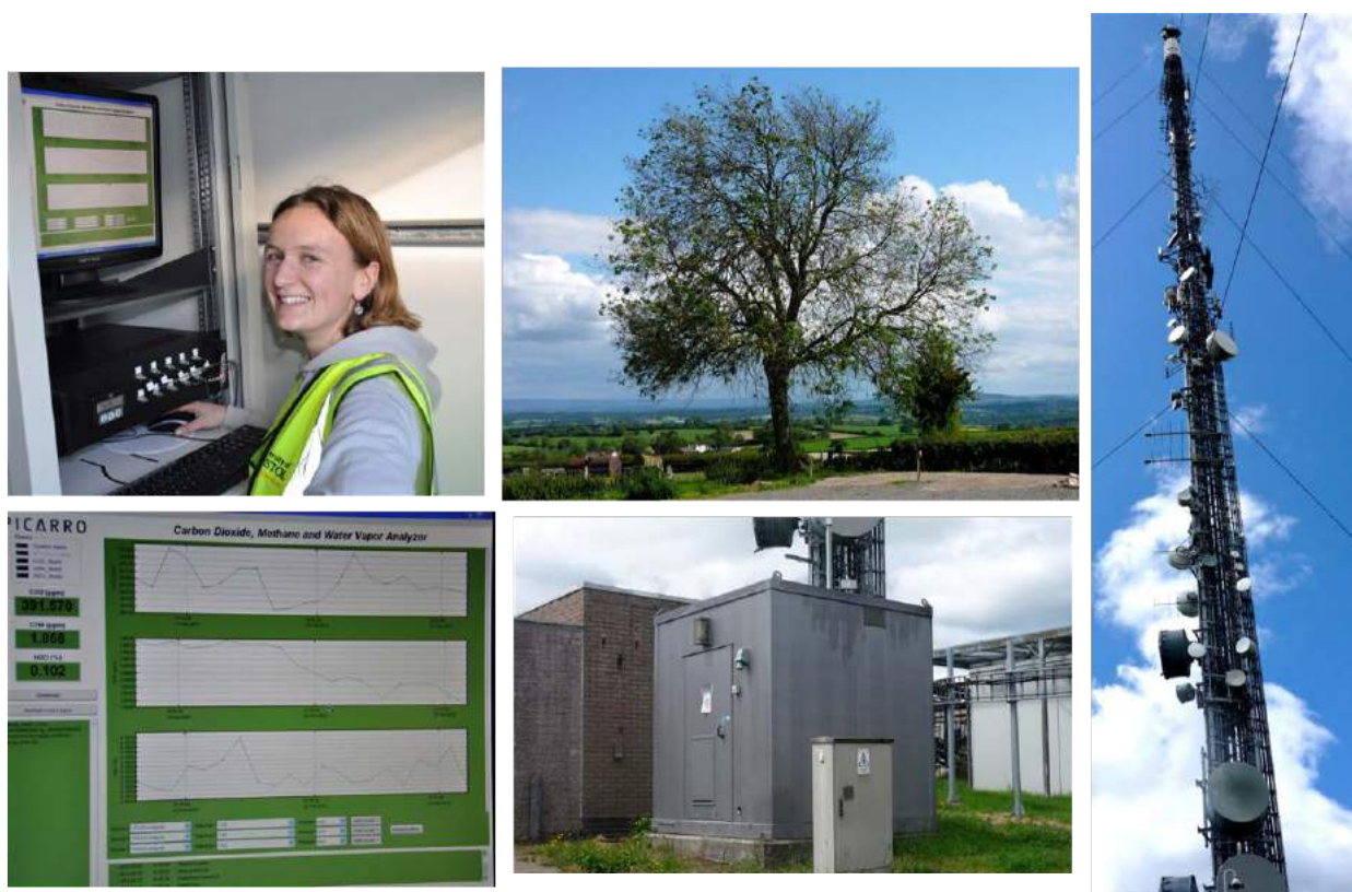
Figure 157: The 166.4 metre Tall tower at Ridge Hill (right) with a view of the surrounding countryside (top centre). The grey cabin houses instrumentation and the images on the left show the first measurements of CO_2 and CH_4 taken from the new site at Ridge Hill.
