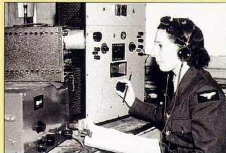
▼ Met. WAAF records signals from a sounding balloon to give measurements of temperature, pressure and humidity in the upper air. © Crown Copyright/MOD
