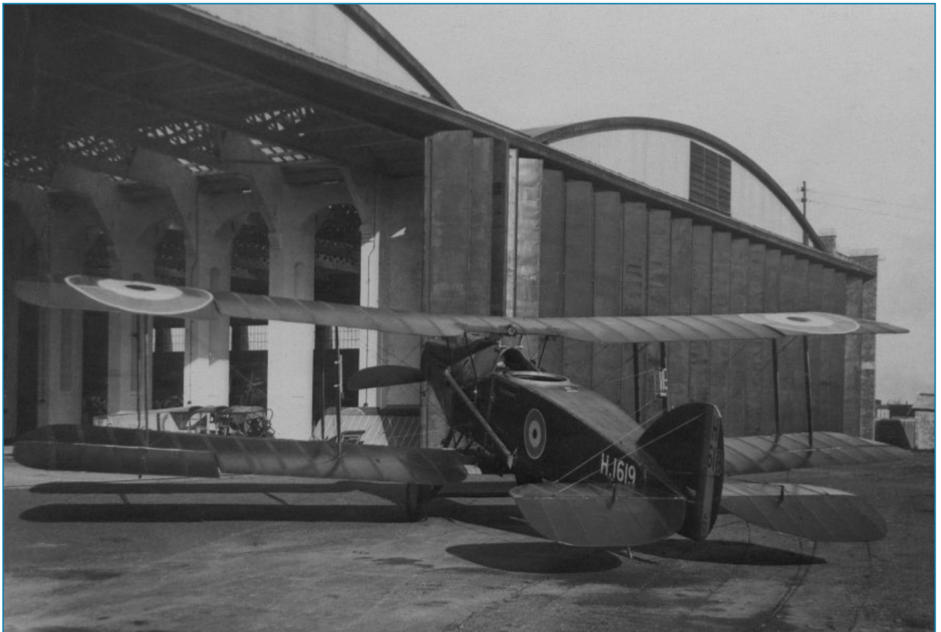
Figure 19. Meteorological flight aircraft Bristol F2b, note the strut psychrometers and lens control wires, circa 1920.
