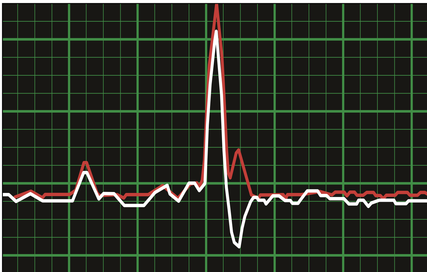
Figure 18. The waveform of a typical sferic. The peak is used for timing.
